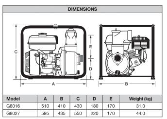
All measurements in mm unless otherwise stated. Above illustration is indicative only for the diesel powered model. Add 1kg for Electric Start engine option.
